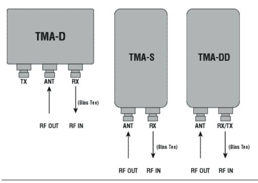
Figure D-1. Tower Mounted Amplifiers
