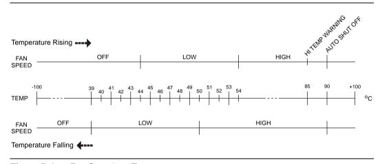
Figure B-3. Fan Speed vs. Temperature
