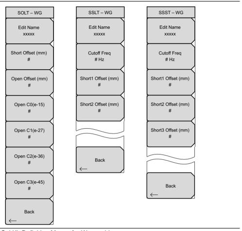
Figure 6-18. Cal Kit Definition Menus for Waveguide
