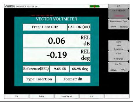
Figure 11-5. Continuous Wave Menu with Relative Measurements
