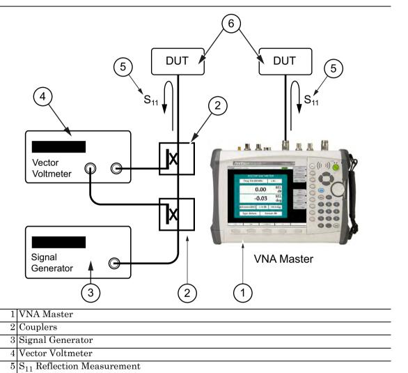
Figure 11-1. Vector Voltmeter within VNA Master
