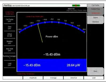
Figure 12-3. Power Meter Display and Cal Factor Menu
