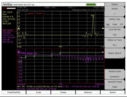
Figure 14-4. Cable with Failing Return Loss (Marker Text Size = Regular)
