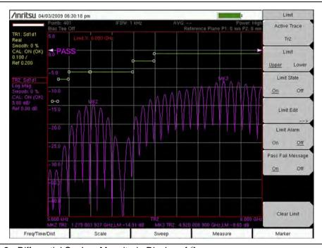
Figure 14-2. Differential  $S_{11}\mbox{ Log}$  Magnitude Display of  $S_{d1d1}$
