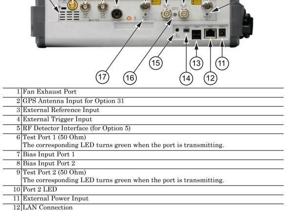
Figure 2-12. MS202xB Test Panel Connectors
