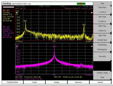
Figure 7-1. Time Domain Measurements of a 3.05 m Cable Showing S<sub>11</sub> and S<sub>21</sub>
