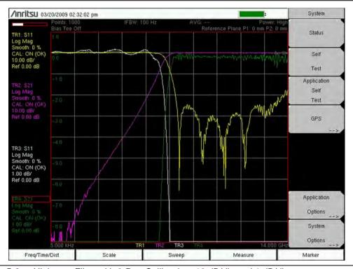
Figure 5-6. Highpass Filter with 2-Port Calibration, 10 dB/div and 1 dB/div
