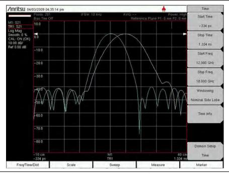
Figure 7-4. S<sub>21</sub> Measurement of 15 cm Long Waveguide Showing Dispersion Compensation
