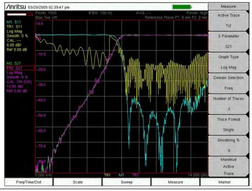
Figure 5-5. High Pass Filter with 2-Port Calibration
