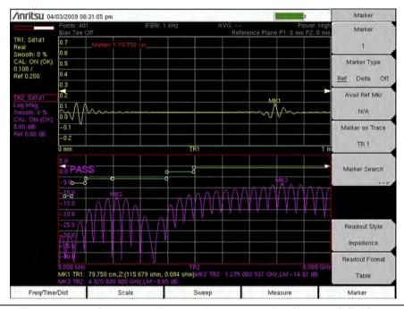
Figure 14-3. Frequency and Distance Domain Responses of Differential Cable
