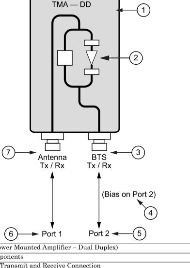
1 TMA-DD (Tower Mounted Amplifier – Dual Duplex)
