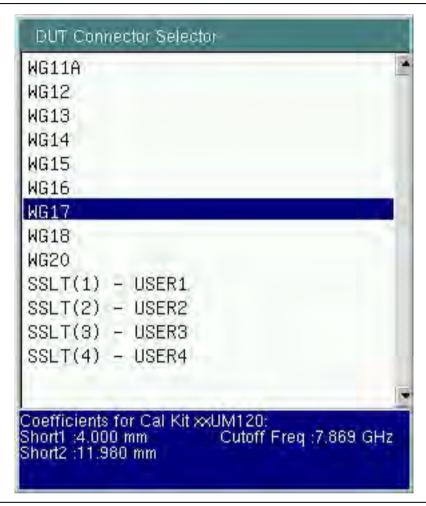
Figure 6-19. DUT Connector Selector List Box for Waveguide
