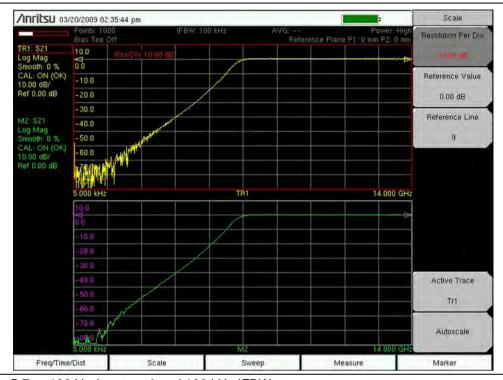
Figure 5-7. 100 Hz (top trace) and 100 kHz IFBW
