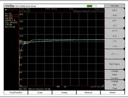
Figure 5-11. Proper Biasing versus Defective Bias Inductor
