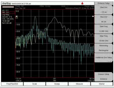
Figure 7-3. S<sub>11</sub> Measurement of 15 cm Long Waveguide Showing Dispersion Compensation
