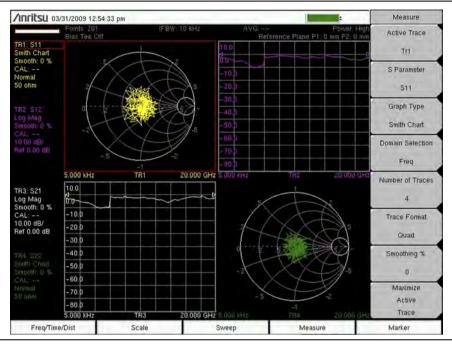
Figure 2-4. 4 Traces in 4 Window Images (Quad Trace Format)
