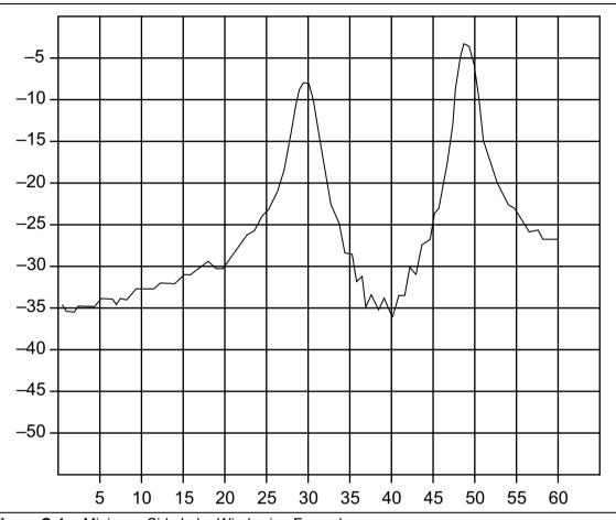
Figure C-4. Minimum Side Lobe Windowing Example
