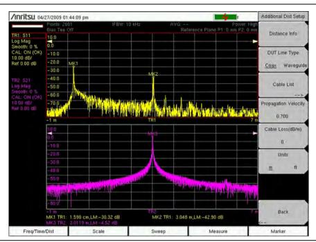
Figure 7-2. Distance Domain Measurements of a 3.05 m Cable Showing S<sub>11</sub> and S<sub>21</sub>
