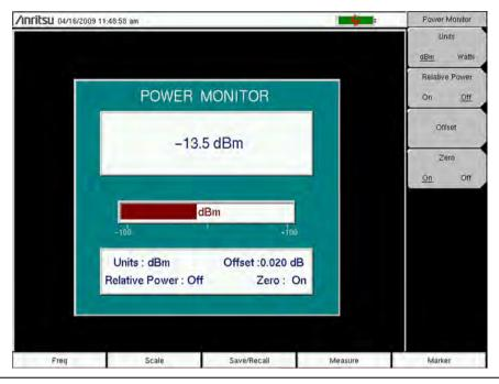
Figure 8-2. Power Monitor Display
