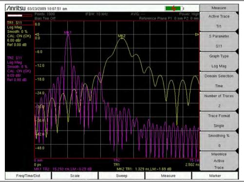
Figure 5-12. S<sub>11</sub> on 15 cm Shorted Waveguide Section
