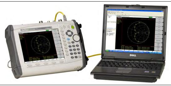
Figure 2-15. MS2028B Connected to PC via Ethernet
