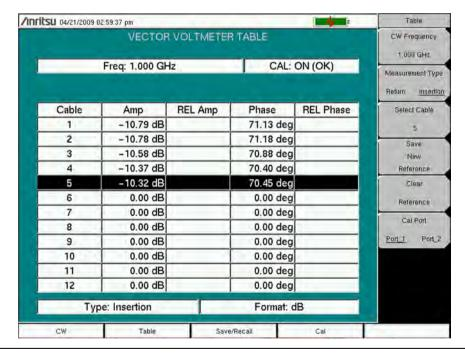
Figure 11-6. Vector Voltmeter Measurement Table
