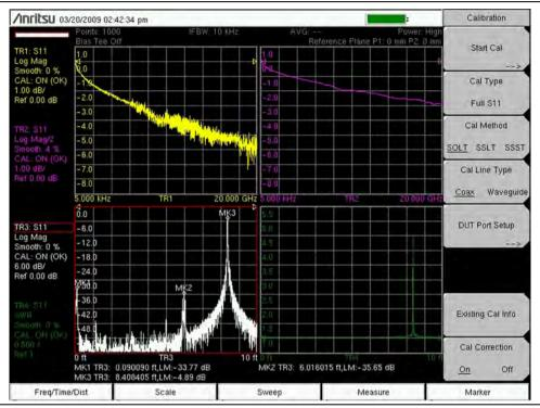
Figure 5-2. Improved Trace with Connector Tightened
