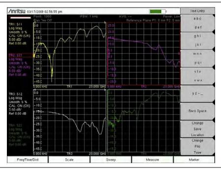
Figure 5-8. Gain, Input Match, Output Match, Isolation of an Amplifier
