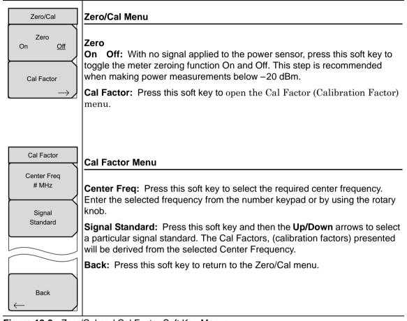
Figure 12-8. Zero/Cal and Cal Factor Soft Key Menus
