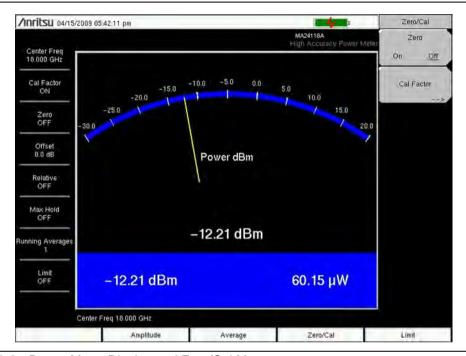
Figure 12-2. Power Meter Display and Zero/Cal Menu
